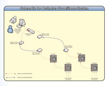
Field controller monitors the operation and intrusion of a specified zone(s) and communicated with CMS located at a distance. Any cutting of cable will immediately trigger alarm at CMS indicationg zone on the PC screen. Graphical representation of the perimeter is depicted on the PC with zones marked on it. Any tampering will be indicated on the PC screen at CMS along with audio siren.
